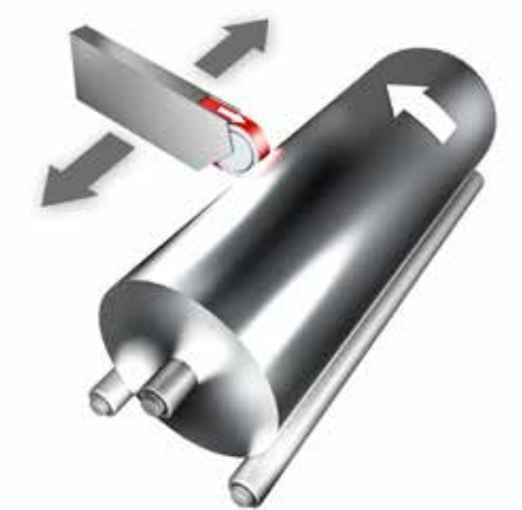
Cylindrical grinding of rollers during roller pass
