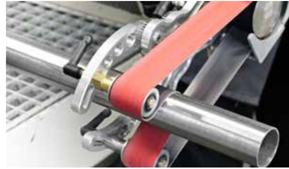
Cylindrical grinding of tubes and bars using hand-held machines
