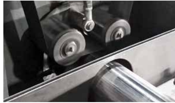
Grinding of longitudinally welded tubes
