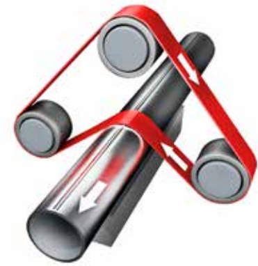
Grinding of longitudinally welded tubes
