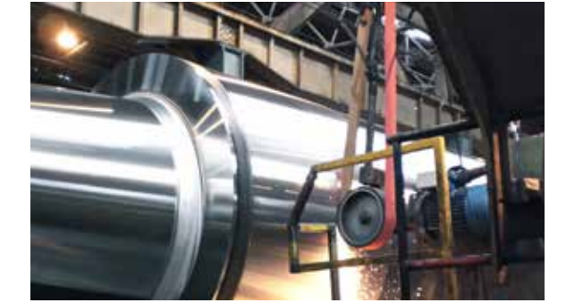
Cylindrical grinding of rollers during roller pass
