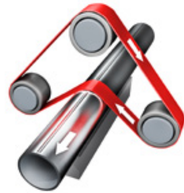
Grinding of longitudinally welded tubes
