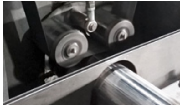
Grinding of longitudinally welded tubes
