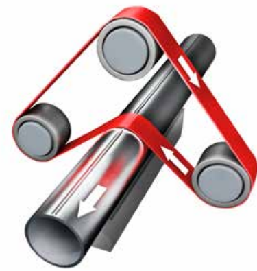
Grinding of longitudinally welded tubes
