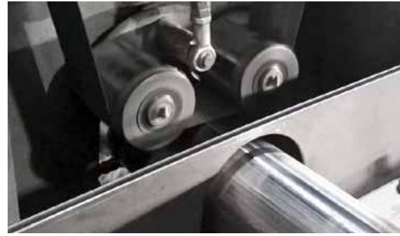
Grinding of longitudinally welded tubes
