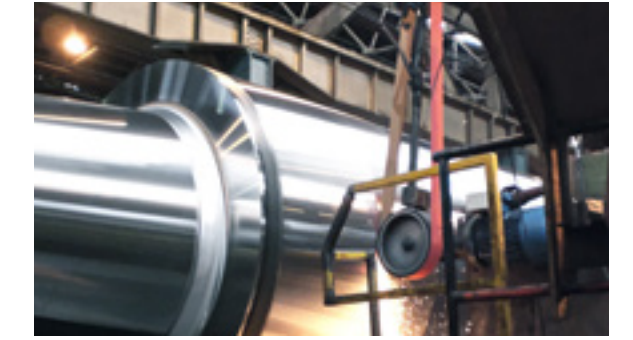
Cylindrical grinding of rollers during roller pass
