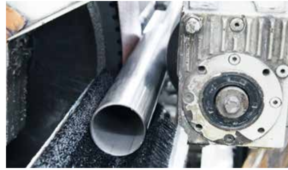
Centerless grinding of tubes and bars
