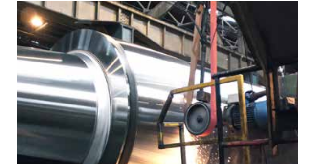
Cylindrical grinding of rollers during roller pass
