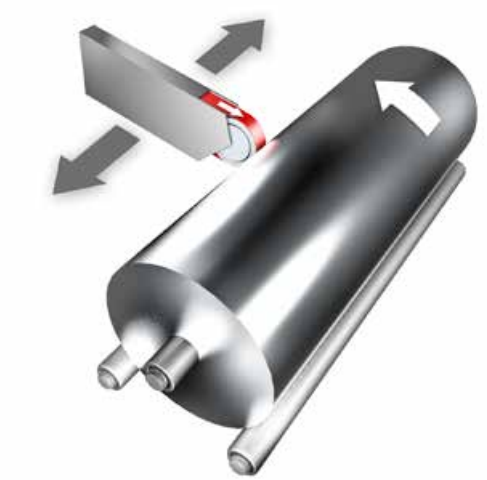
Cylindrical grinding of rollers during roller pass
