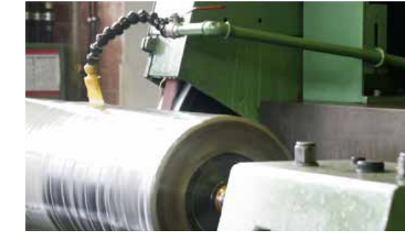
Cylindrical grinding of piston rods and cylinders and grinding between centres
